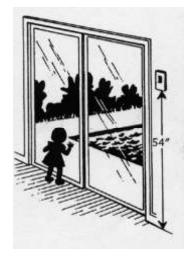
Doors with direct access to the pool must be equipped with alarms meeting Appendix G requirements (alarms meeting UL 2017 are acceptable). Door alarms associated with home security systems will not usually meet these requirements. This does "NOT" replace the requirement for Pool Barriers.
