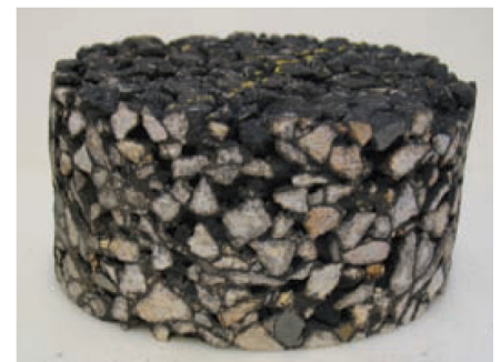
Pervious pavement allows water infiltration and reduction in winter road sand and salt necessary to keep roads clear.
